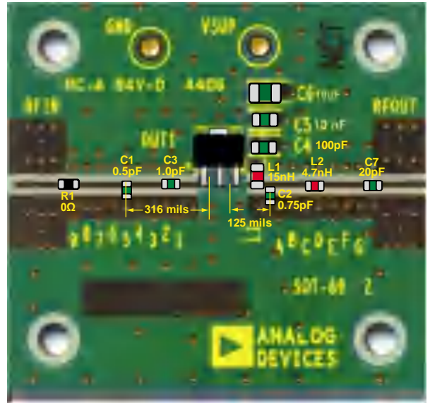
Figure 47. Evaluation Board Layout and Component Placement, 3500 MHz to 3700 MHz Operation
