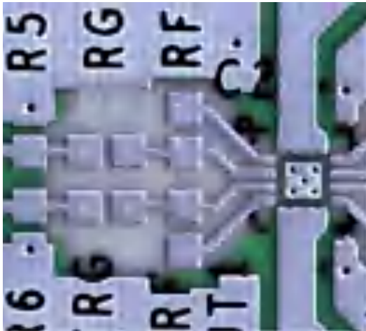
Figure 51. Ground and Power Plane Voiding in Vicinity of R_F and R_G
