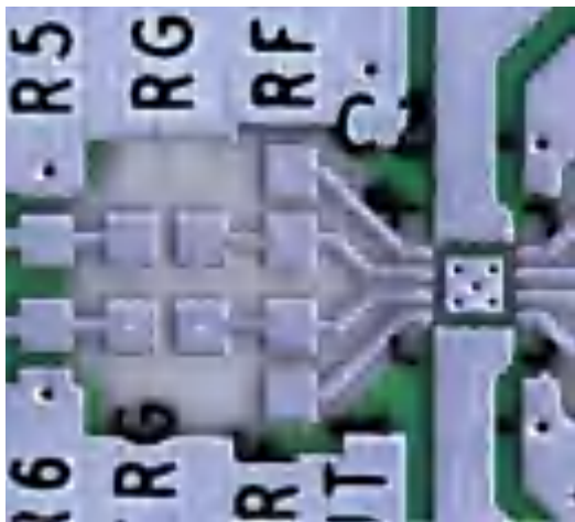
Figure 56. ADA4930-1 Ground and Power Plane Voiding in the Vicinity of R_F and R_G
