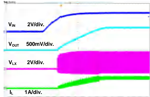
Figure 11. Power On through VIN Waveform
